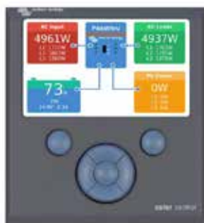
Color Control GX, showing a PV application
